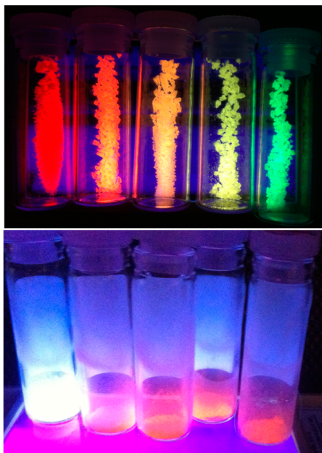
Figure 3. (Top) Photoluminescence of [\text{Bu}_4\text{N}]_2[\text{Eu}_x\text{Tb}_{1-x}(\text{NO}_3)_4\text{Au}(\text{CN})_2] using a long wavelength UV-lamp excitation source at room temperature; from left to right x = 1, 0.75, 0.50, 0.25, 0 , illustrating color tuning ability. (Bottom) Photoluminescence of \text{Eu}_x\text{Tb}_{1-x}[\text{Au}(\text{CN})_2]_3 \cdot 3\text{H}_2\text{O} using a long wavelength UV-lamp excitation source at 77 K; from left to right x = 0, 0.25, 0.50, 0.75, 1 , illustrating the energy transfer resulting in only europium-based emission.
